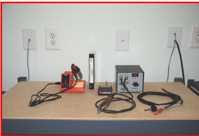
Photo One (Left to Right) Weller Soldering Station (5-40 Watts) (Temperatures to 900 degrees F)
